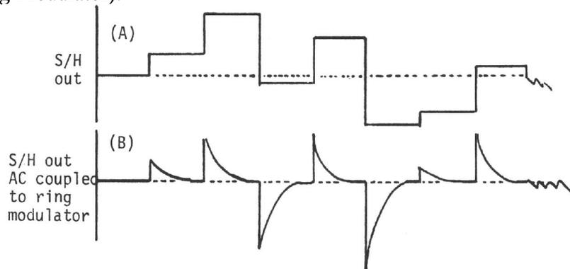
8. If the other signal input to the Ring Modulator carries an audio-frequency signal, that signal will be modulated by the voltage fluctuations of 7b above to produce a series of "events":
