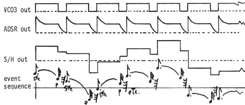
The diagram should make clear why this is happening. Changing the pulse-width now will change the rhythmic "feel" of the pitch-sequence. The second pitch in each envelope can be made to "disappear" by shortening the final decay (i.e. "release") time or by shortening the pulse-width to minimum. (There is at least one other way of doing this; figure it out and send us a note about it.)
